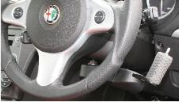
Single lever accelerator and brake – here fitted with optional indicator switch – Jeff Gosling
